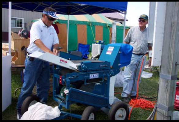
John Oughterson and Bill Garman processing Brassica seed using the belt thresher.
